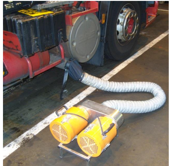
Above: dual L20 filters with flexible hose & sock adapter
